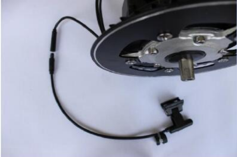
Step 4: the vehicle speed sensor and the motor home plug inserted;
